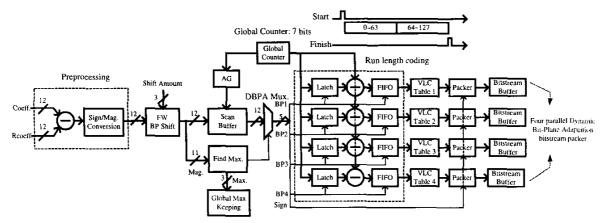
Figure 3. Proposed block-level processing core for FGS encoder.
